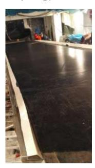
Shaw Almex's unique vulcanization plate, pressure bag and temperature control box can ensure uniform pressure in the curing area so that the optimal joint can be vulcanized.
